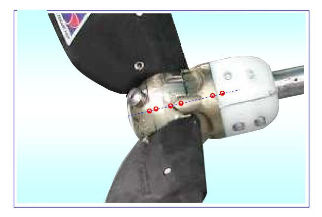
WARNING: Customers are strongly advised not to attempt to disassemble the unit unless this becomes absolutely essential. Re-assembly of all the components coupled with the need to ensure sealant is inserted into the nose cone whilst at the same time preloading the internal torsion spring makes for a tricky operation, particularly if no stub shaft is available to hold the unit whilst these operations are completed.
